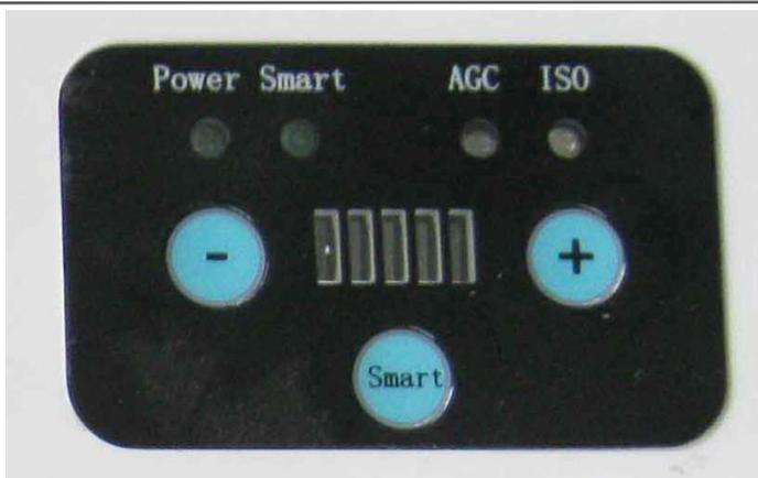
Figure 3 Front panel of the repeater
